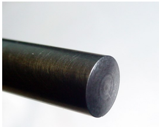
Photo – 4 Push Rod Exhibiting Normal Wear
