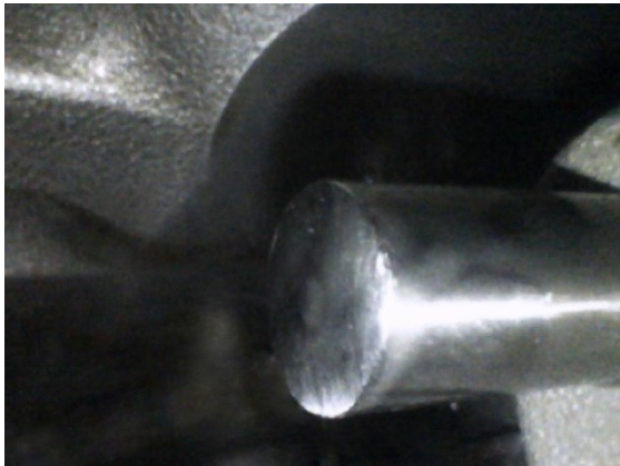
Photo – 3 Damaged Push Rod
