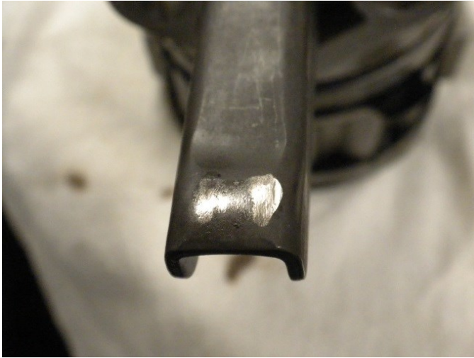
Photo – 1 Damaged Pump Lever
