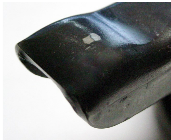
Photo – 2 Pump Lever Exhibiting Normal Wear
