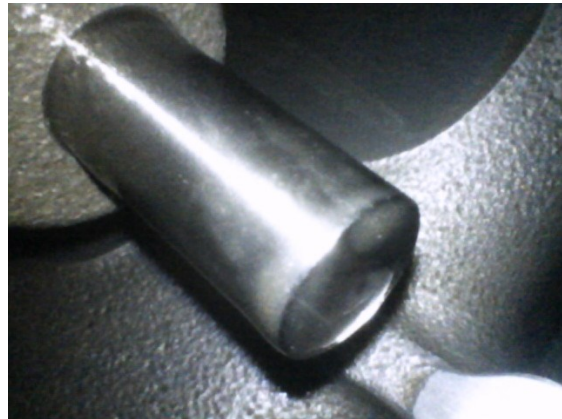
Photo – 3 Damaged Push Rod
