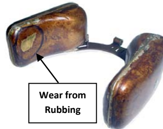
Example: Wear from Rubbing on Large MA Float
